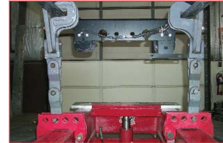
HOLD DOWNS ARE EASILY MADE BY LINKS AND PINS. SLACK IS REMOVED BY LOWERING THE FRAME PRESS, THEN PRESSURE IS APPLIED.
