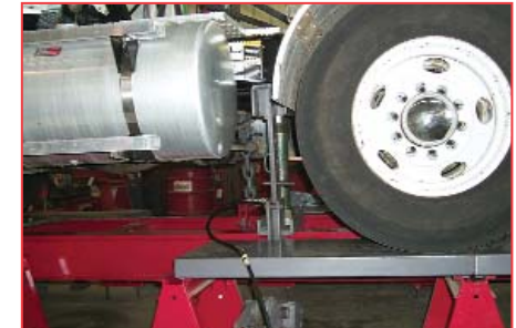
THIS TWIST CORRECTION SET UP CAN BE PERFORMED WITHOUT REMOVING THE FUEL TANK.
