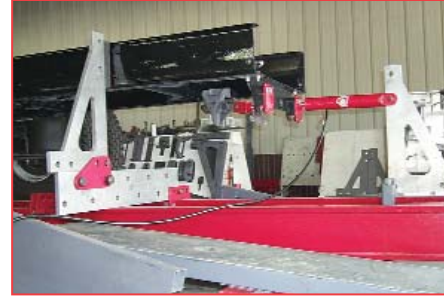
THIS DIAMOND CORRECTION SET UP UTILIZES THE FORCE OF A PULL RAM TO BRING THE FRAME RAILS EVEN WITH EACH OTHER.
