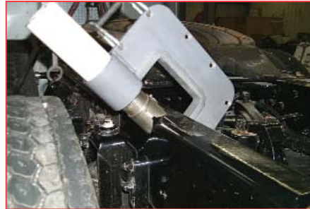
THIS 20 TON C CLAMP CORRECTS THE RADIUS OF A FRAME. INTERCHANGEABLE C CLAMP TOOLING HEADS ALLOW IT TO CORRECT THE SMALLEST IMPERFECTION.
