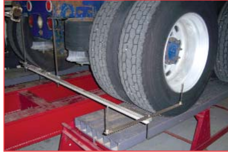
A DIAMOND SIGHT GAUGE ATTACHES TO THE REAR-MOST FRAME GAUGE AND DIAGNOSES DIAMOND FRAME CONDITIONS.
