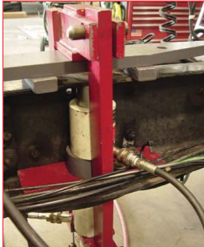
OUR FLANGE PRESS SAFELY REMOVES IMPERFECTIONS TO THE FRAME WITH A HYDRAULIC RAM.
