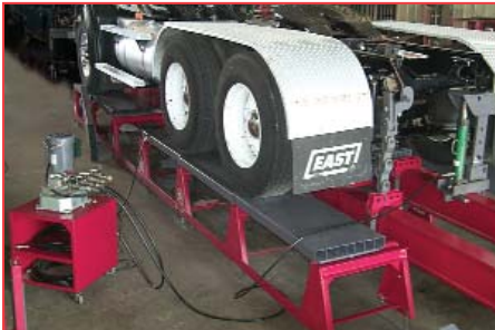
THIS TWIST SET UP IS BEING POWERED BY THE BEE LINE 900B 4 VALVE HYDRAULIC PUMP.
