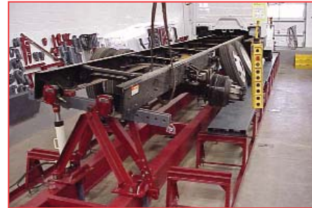
A TWIST IN AN EXTRA LONG TRACTOR FRAME CAN BE CORRECTED WITH OUR TRAILER TWISTING TOOLS.
