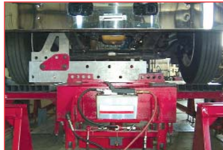
THIS HOLD ON A SIDE SWAY SET UP IS POSITIONED AGAINST THE FRAME RAIL WITHOUT THE FRONT WHEELS BEING REMOVED.
