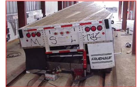
THIS TWISTED TRAILER IS BEING CORRECTED WITH OUR TRAILER TWISTING TOOLS. OUR FLOOR "I" BEAM SET UP WORK PRIMARILY WITH TRAILER CORRECTIONS.
