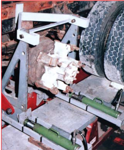
THIS REAR AXLE BYPASS SET UP IS CRITICAL IN MAKING PUSHES TO PINPOINTED AREAS WITHOUT REMOVING THE AXLE.
