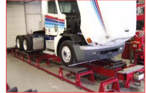
FRAME GAUGING AND EQUIPMENT SET UP IS DONE AT A CONVENIENT HEIGHT. RUNWAYS CAN BE REMOVED TO ALLOW EASY ACCESS.
