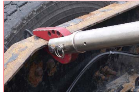
A HAND FLANGE TOOL MAKES CORRECTIONS TO IMPERFECTIONS IN BEAMS. AN EXTENDABLE HANDLE PROVIDES LEVERAGE FOR THE CORRECTION.
