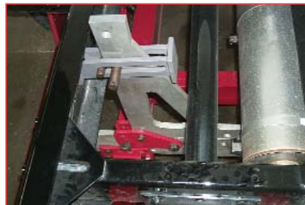
EXTRA CLEARANCE CAN BE ADDED TO OUR LIGHTWEIGHT ALUMINUM KNEES TO MAKE DIRECT HOLDS ON THE FRAME RAIL.
