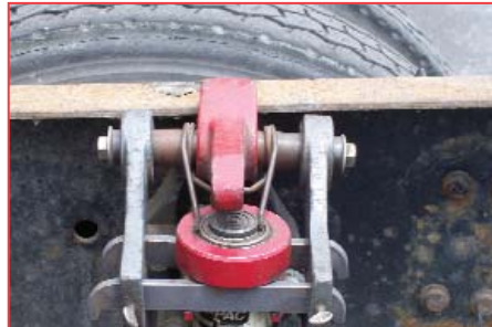
THE 1420 FLANGE FINISHER UTILIZES THE FORCE OF THE 10 TON RAM TO EASILY FINISH BEAMS UP TO 1/2" THICK.
