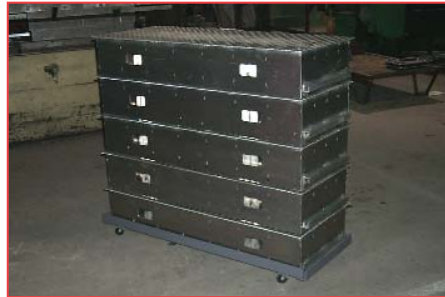
BEE LINE ALUMINUM RUNWAYS COMPLIMENT TO THE PORTABLE FRAME PRESS. STACKABILITY INSURES VEHICLE SUPPORT WHILE MAKING CORRECTIONS. (ABOVE LEFT)
