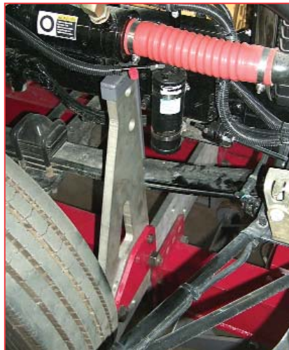
THIS SET UP FEATURES AN ALUMINUM KNEE TOPPED WITH A BEE LINE KNEE PROTECTOR THAT INSURES FLUSH CONTACT WITH THE FRAME RAIL.
