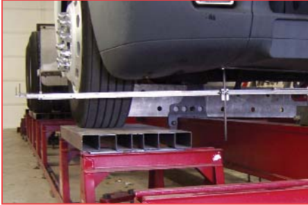
OUR SELF CENTERING FRAME GAUGES EXTEND THE CENTERLINE TO THE OUTSIDE OF THE CHASSIS FOR EASY DIAGNOSIS OF MISALIGNMENT CONDITIONS.
