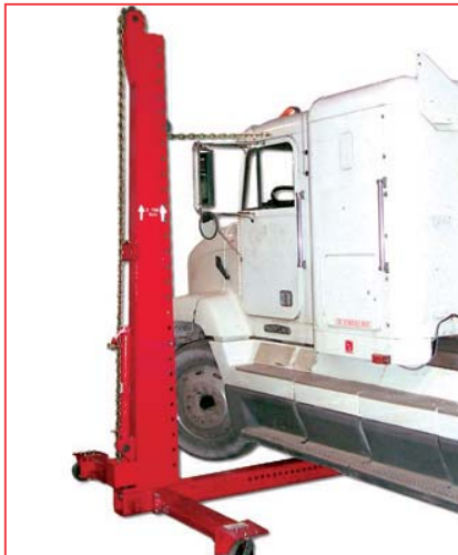
THE BEE LINE POWER TOWER IS AN EXCELLENT TOOL TO COMPLIMENT OUR FRAME PRESS. HIGH CAB OR TRAILER PULLS CAN BE MADE WITH GREAT FORCE.
